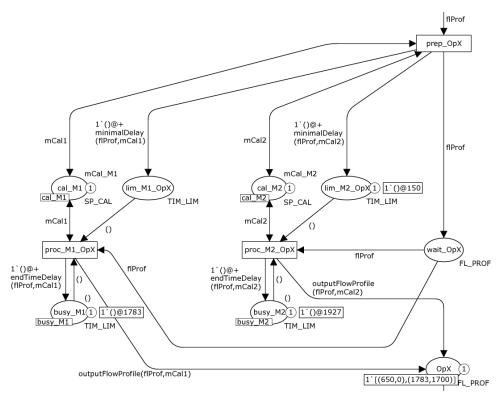
Fig. 8. Execution of the Petri net model – the state after execution of the transition proc\_M1\_OpX
