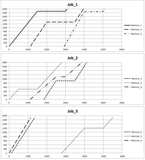
Fig. 10. The result of the production system simulation - the output flow profiles plot
