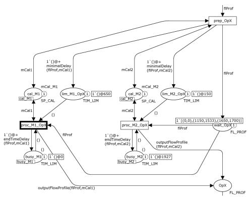
Fig. 7. Execution of the Petri net model – the state after execution of the transition  $prep_OpX$
