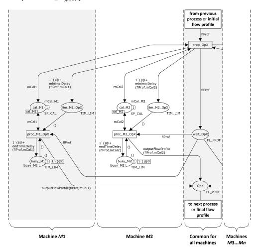
Fig. 6. The Petri net model substructure that represents one operation
